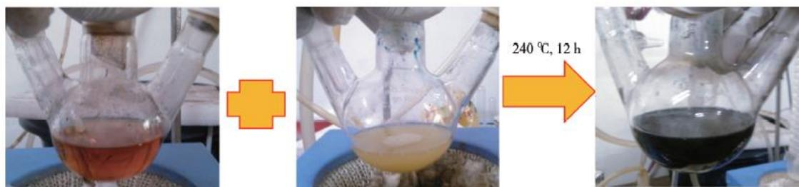
Fig. 6. Synthesis process of CZTS nanoparticles in hot injection method
